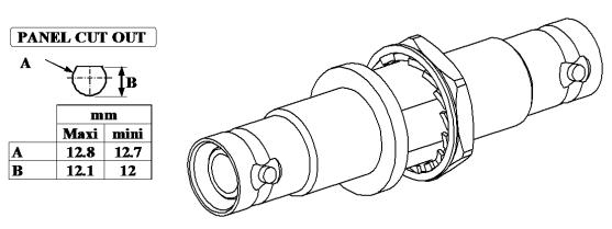
All dimensions are in mm. Tolerances according ISO 2768 m-H
