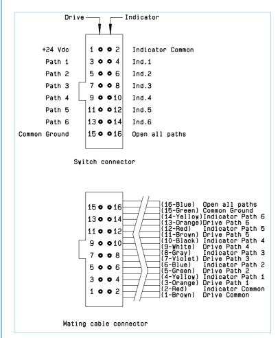
Ways 1 and 4 are not connected for SP4T switches.
