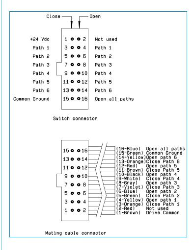
Ways 1 and 4 are not connected for SP4T switches.
