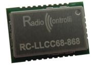
LoRa Smart Home (LLCC68) is a sub-GHz LoRa® RF Transceiver for medium range indoor and indoor to outdoor wireless applications. SPI interface. Designed for long battery life with just 4.2 mA of active receive current consumption. The LLCC68 can transmit up to +22 dBm with highly efficient integrated power amplifiers.
