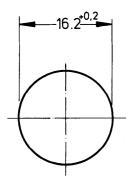
PCB hole pattern, sight on component side
