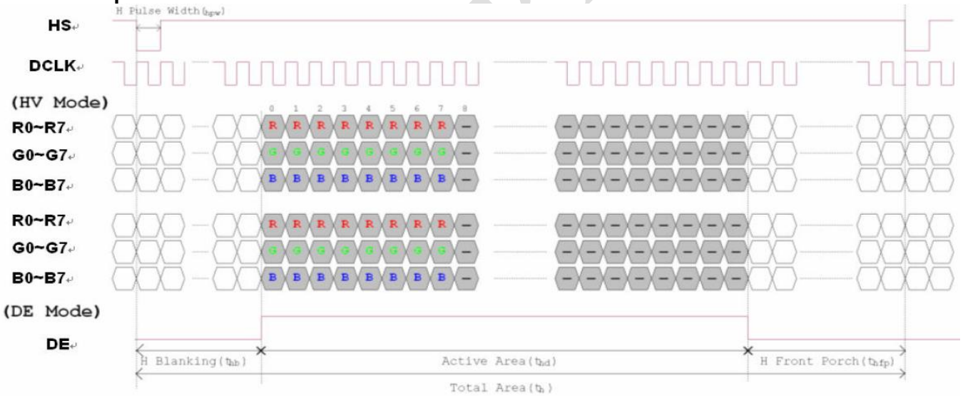
Fig. Horizontal input timing diagram
