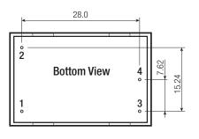
Allow 5mm clearance around converter for air circulation
