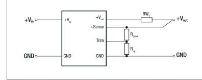
The output voltage can be adjusted via the trim and sense functions. The maximum output voltage from Trim and Sense
