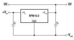
$\mathbf{C_1}$  and  $\mathbf{C_2}$  may be added to reduced ripple and should be fitted close to the converter pins.
