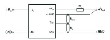
The output voltage can be adjusted via the trim and sense functions.
