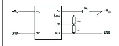
The output voltage can be adjusted via the trim and sense functions.
