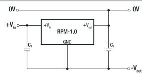
$\mathbf{C}_{1}$  and  $\mathbf{C}_{2}$  may be added to reduced ripple and should be fitted close to the converter pins.
