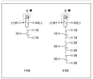
${\pmb 0}$  The control terminal S is activated by connection to A1 terminal via the external control contact S.
