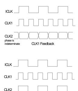
Using CLK1 as feedback will always result in synchronized rising edges between ICLK and CLK1 if CLK1 is used as feedback. CLK2 could be a falling edge compared to ICLK. Therefore, wherever possible, it is recommended to use CLK2 for feedback, which will synchronize the rising edges of all three clocks.
