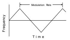
Modulation Frequency = Input Frequency/10000
