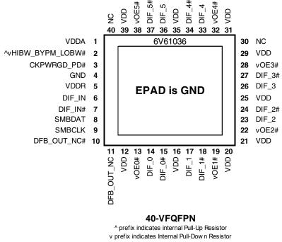
^v prefix indicates Interal Pull-Up/Dow n Resistor (biased to \$VDD/2\$)
