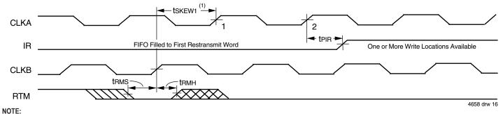
1. tskew1 is the minimum time between a rising CLKB edge and a rising CLKA edge for IR to transition HIGH in the next CLKA cycle. If the time between the rising CLKB edge and rising CLKA edge is less than tskew1, then IR may transition HIGH one CLKA cycle later than shown.
