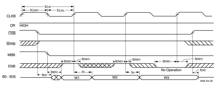
Figure 6. FIFO Read Cycle Timing
