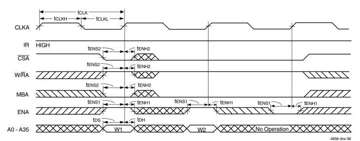
Figure 5. FIFO Write Cycle Timing
