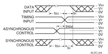
Set-up, Hold, and Release Times
