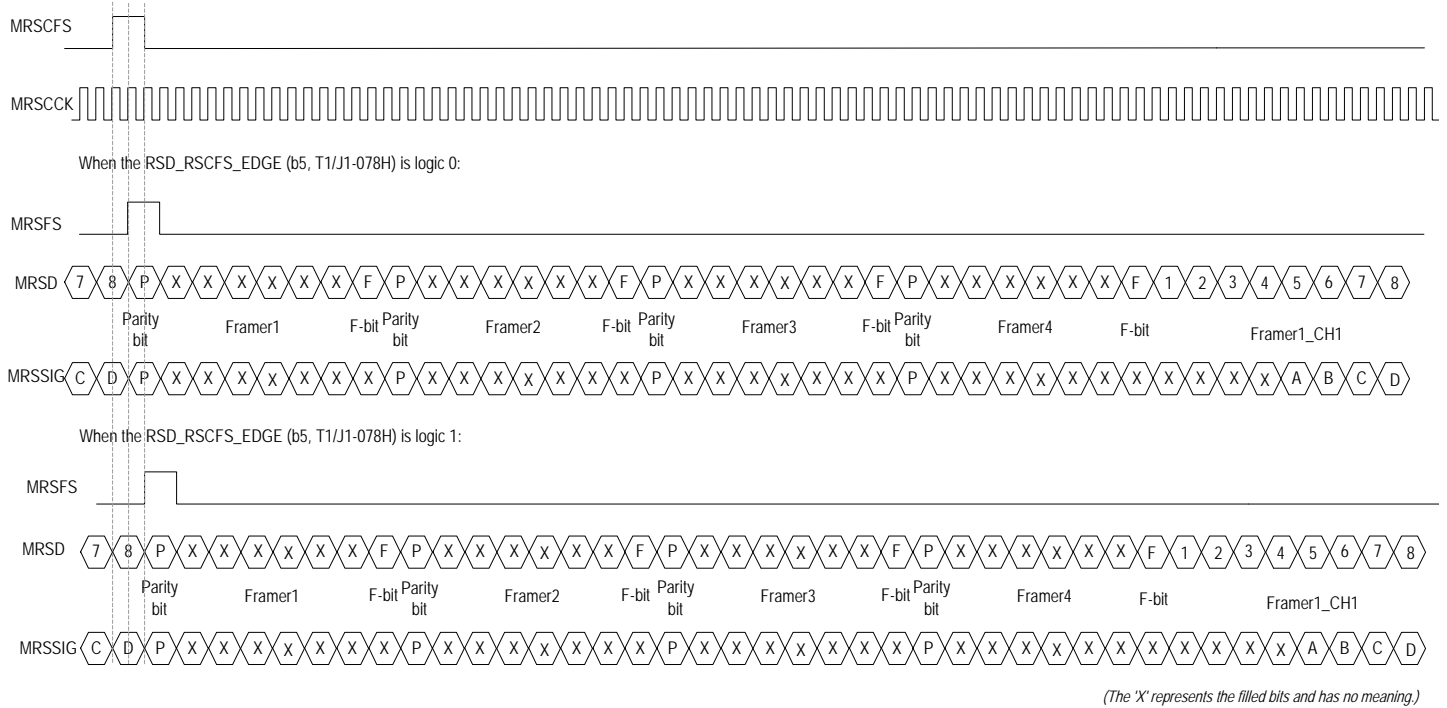
Figure 34. T1/J1 Receive Multiplexed Mode - Functional Timing Example 2
