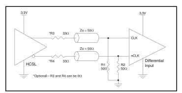
Figure 2E. HiPerClockS CLK/nCLK Input Driven by a 3.3V HCSL Driver
