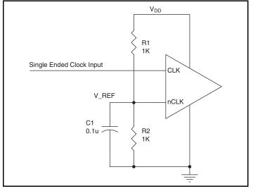
Figure 1. Single-Ended Signal Driving Differential Input
