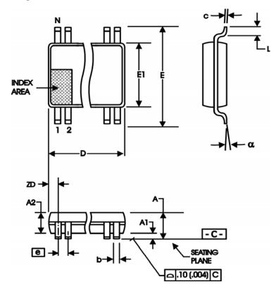
Table 7. Package Dimensions for 28 Lead SSOP
