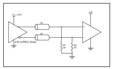
Figure 4C. 2.5V LVPECL Driver Termination Example
