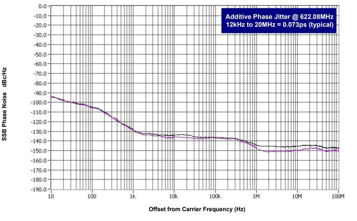
As with most timing specifications, phase noise measurements has issues relating to the limitations of the equipment. Often the noise floor of the equipment is higher than the noise floor of the device. This is illustrated above. The device meets the noise floor of what is shown, but can actually be lower. The phase noise is dependent on the input source and measurement equipment.
