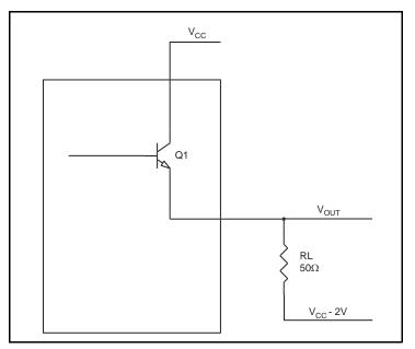
Figure 5. LVPECL Driver Circuit and Termination
