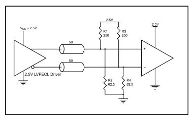
Figure 4A. 2.5V LVPECL Driver Termination Example
