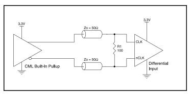
Figure 2B. HiPerClockS CLK/nCLK Input Driven by a Built-In Pullup CML Driver
