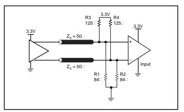
Figure 3B. 3.3V LVPECL Output Termination
