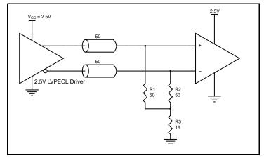
Figure 4B. 2.5V LVPECL Driver Termination Example
