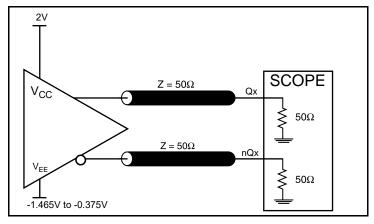
LVPECL Output Load AC Test Circuit
