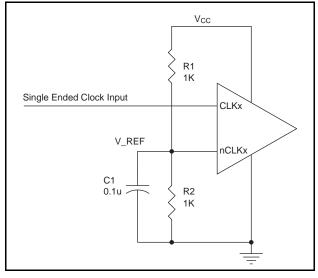
Figure 1. Single-Ended Signal Driving Differential Input
