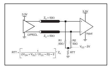
Figure 3A. 3.3V LVPECL Output Termination
