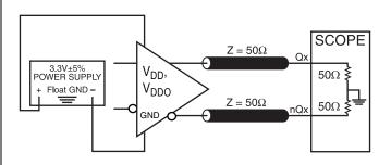
Figure 3. 2.5V Core/ 2.5V Output Load AC Test Circuit
