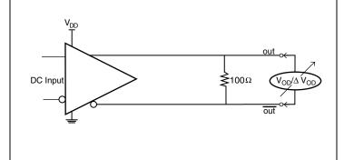
Figure 11. Offset Voltage Setup
