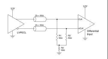
Figure 15. CLK/ nCLK Input Driven by a 3.3V LVPECL Driver
