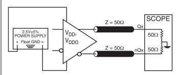
Figure 4. Differential Input Level
