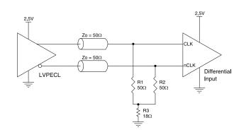
Figure 21. CLK/ nCLK Input Driven by a 2.5V LVPECL Driver
