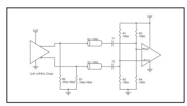
Figure 2B. PCLK/nPCLK Input Driven by a 2.5V LVPECL Driver with AC Couple
