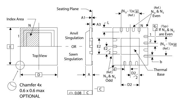
THERMALLY ENHANCED, VERY THIN, FINE PITCH QUAD FLAT / NO LEAD PLASTIC PACKAGE
