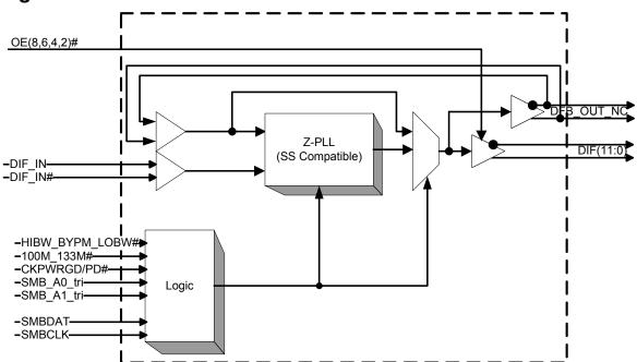
IDT® 12-OUTPUT LOW POWER DIFFERENTIAL BUFFER FOR PCIE GEN3 AND QPI
