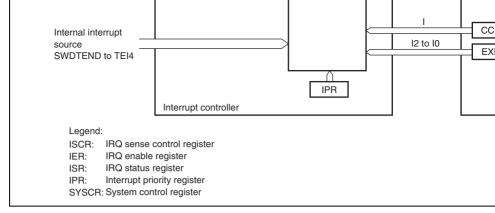
Figure 5.1 Block Diagram of Interrupt Controller
