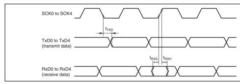
Figure 24.22 SCI Input/Output Timing/Synchronous Mode
