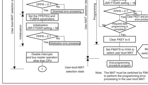
Figure 20.14 Procedure for Programming User MAT in User Boot Mod
