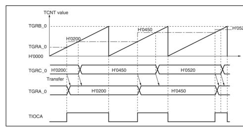
Figure 10.15 Example of Buffer Operation (1)
