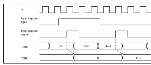
Figure 10.33 Input Capture Input Signal Timing
