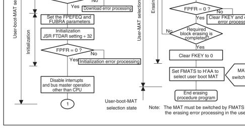
Figure 20.15 Procedure for Erasing User MAT in User Boot Mode
