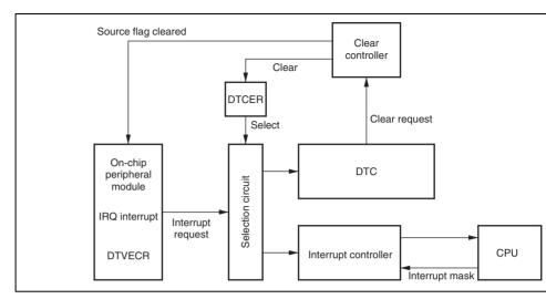
Figure 8.2 Block Diagram of DTC Activation Source Control
