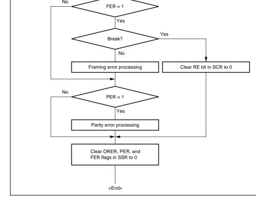
Figure 13.9 Sample Serial Reception Data Flowchart (2)
