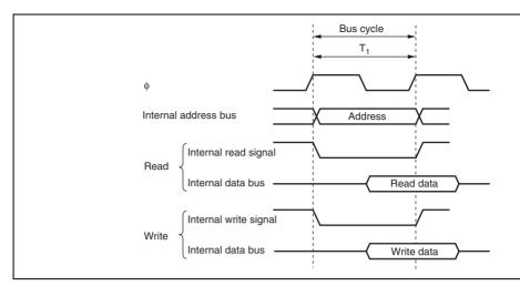
Figure 7.4 On-Chip Memory Access Cycle
