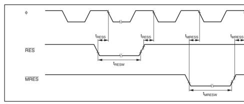
Figure 24.7 Reset Input Timing
