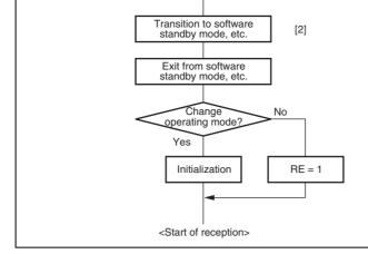
Figure 13.37 Sample Flowchart for Mode Transition during Reception
