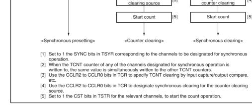
Figure 10.10 Example of Synchronous Operation Setting Procedure
