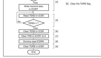
Figure 14.19 Sample Flowchart for Slave Transmit Mode
