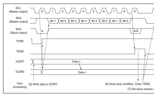
Figure 14.6 Master Transmit Mode Operation Timing (2)
