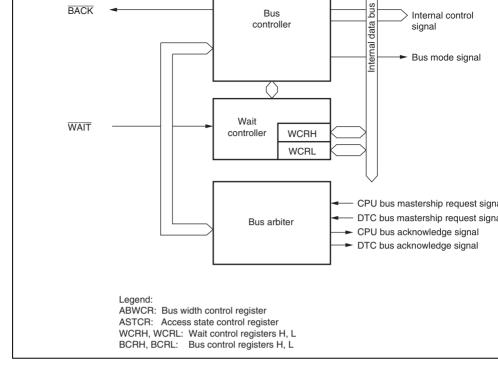
Figure 7.1 Block Diagram of Bus Controller
