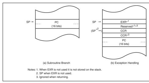
Figure 2.2 Stack Structure in Normal Mode
