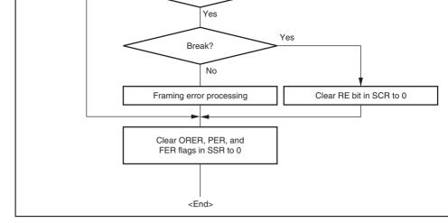
Figure 13.13 Sample Multiprocessor Serial Reception Flowchart (2)
