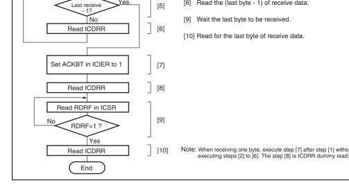
Figure 14.20 Sample Flowchart for Slave Receive Mode
