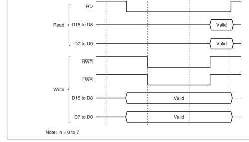
Figure 7.23 Bus Timing for 16-Bit 3-State Access Space (3) (Word Access)
