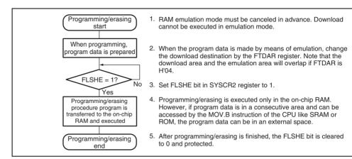
Figure 20.9 Programming/Erasing Overview Flow
