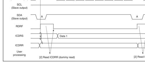
Figure 14.11 Slave Receive Mode Operation Timing (1)
