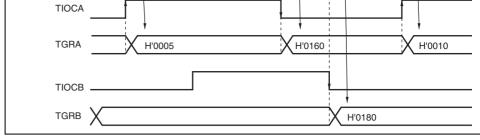
Figure 10.9 Example of Input Capture Operation
