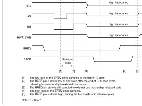
Figure 7.30 Bus Mastership Released State Transition Timing
