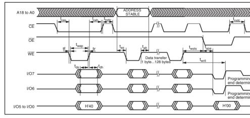
Figure 20.33 Waveform of Automatic Programming Mode
