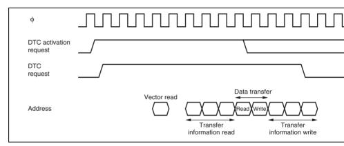
Figure 8.10 DTC Operation Timing (Example in Normal Mode or Repeat Mo
