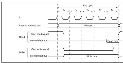
Figure 7.12 On-Chip HCAN Module Access Cycle
