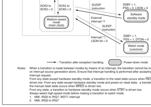
Figure 22.1 Mode Transition Diagram
