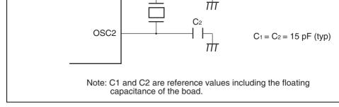
Figure 21.8 Connection Example of 32.768-kHz Crystal Resonator
