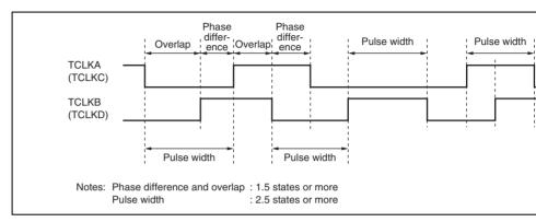
Figure 10.44 Phase Difference, Overlap, and Pulse Width in Phase Counting
