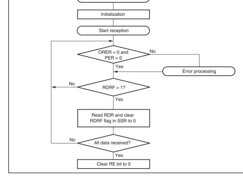
Figure 13.30 Example of Reception Processing Flow
