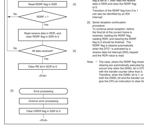
Figure 13.19 Sample Serial Reception Flowchart
