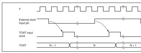
Figure 11.4 Count Timing for External Clock Input
