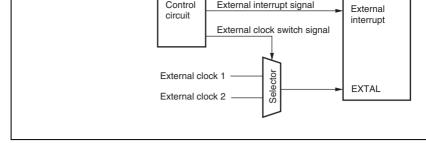
Figure 21.6 External Clock Switching Circuit (Examples)
