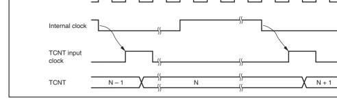
Figure 11.3 Count Timing for Internal Clock Input
