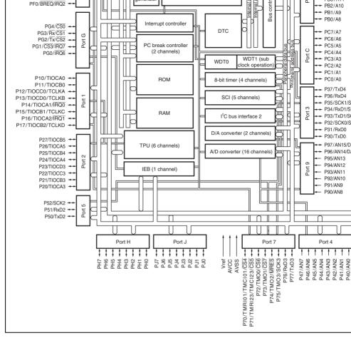
Figure 1.2 Internal Block Diagram of H8S/2552 Group
