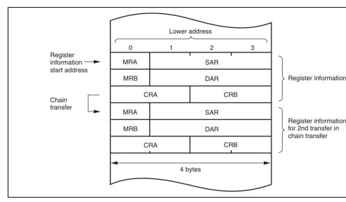
Figure 8.3 Location of DTC Register Information in Address Space
