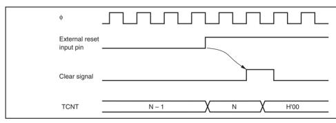
Figure 11.8 Timing of Clearing by External Reset Input
