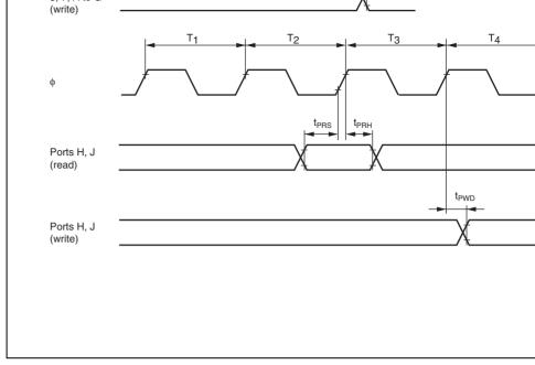
Figure 24.14 I/O Port Input/Output Timing
