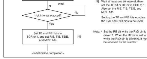
Figure 13.5 Sample SCI Initialization Flowchart
