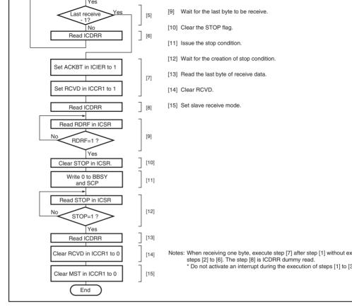
Figure 14.18 Sample Flowchart for Master Receive Mode
