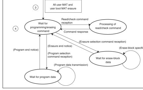
Figure 20.8 Overview of Boot Mode State Transition Diagram
