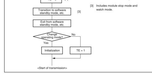
Figure 13.34 Sample Flowchart for Mode Transition during Transmission
