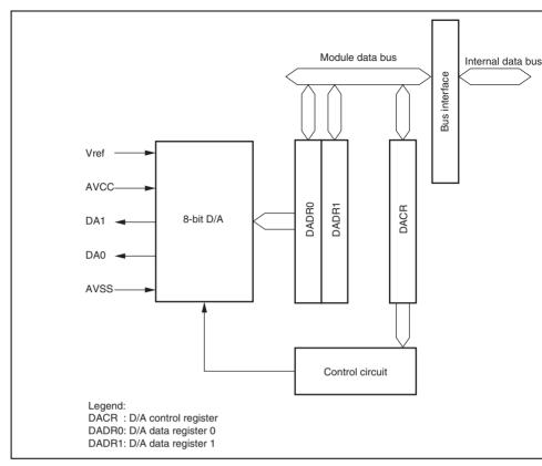
Figure 16.1 Block Diagram of D/A Converter
