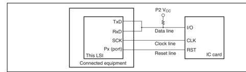
Figure 13.21 (1) Schematic Diagram of Smart Card Interface Pin Connecti (Channels 0, 1, 3, and 4)
