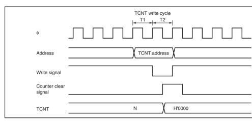
Figure 10.45 Contention between TCNT Write and Clear Operations
