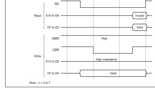
Figure 7.22 Bus Timing for 16-Bit 3-State Access Space (2) (Odd Address Byte
