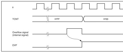
Figure 12.4 Timing of OVF Setting
