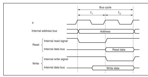
Figure 7.6 On-Chip Peripheral Module Access Cycle
