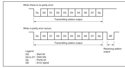
Figure 13.22 Normal Smart Card Interface Data Format
