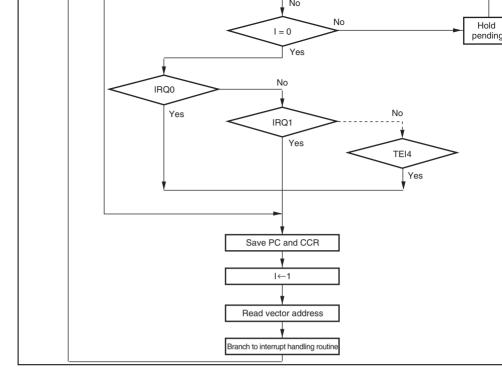
Figure 5.5 Flowchart of Procedure up to Interrupt Acceptance in Interrupt Control Mode 0
