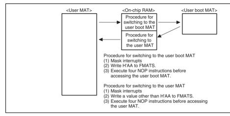
Figure 20.20 Switching between the User MAT and User Boot MAT
