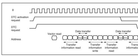
Figure 8.12 DTC Operation Timing (Example of Chain Transfer)
