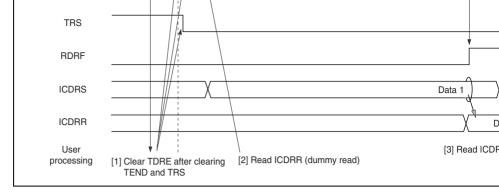
Figure 14.7 Master Receive Mode Operation Timing (1)
