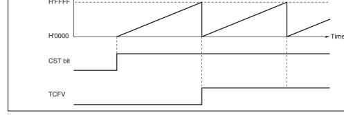
Figure 10.3 Free-Running Counter Operation
