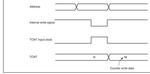
Figure 12.8 Contention between TCNT Write and Increment
