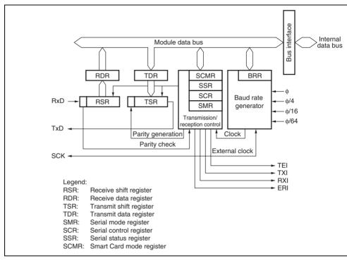
Figure 13.1 Block Diagram of SCI
