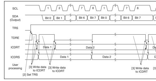
Figure 14.14 Transmit Mode Operation Timing
