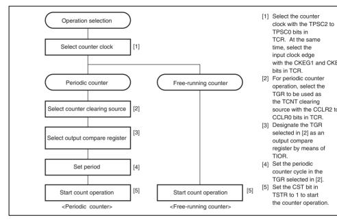
Figure 10.2 Example of Counter Operation Setting Procedure
