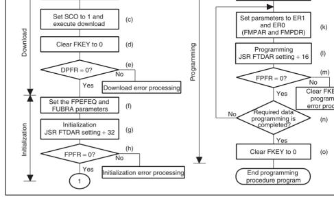
Figure 20.11 Programming Procedure
