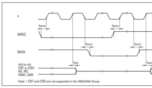
Figure 24.13 External Bus-Released Timing
