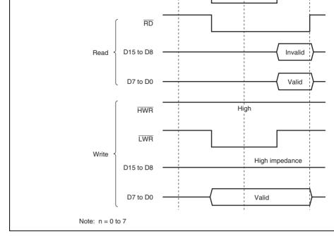
Figure 7.19 Bus Timing for 16-Bit 2-State Access Space (2) (Odd Address Byte A
