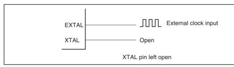
Figure 21.4 External Clock Input (Examples)
