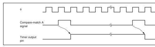
Figure 11.6 Timing of Timer Output
