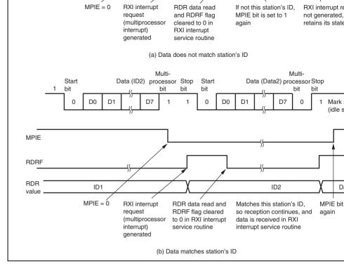
Figure 13.12 Example of SCI Operation in Reception (Example with 8-Bit Data, Multiprocessor Bit, One Stop Bit)
