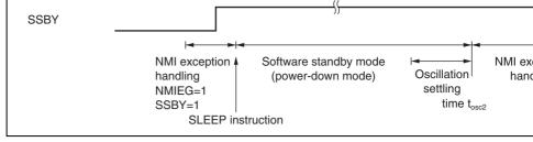
Figure 22.3 Software Standby Mode Application Example
