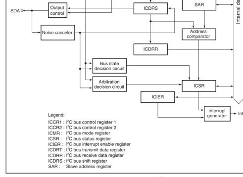
Figure 14.1 Block Diagram of I<sup>2</sup>C Bus Interface 2
