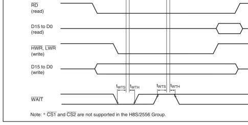
Figure 24.11 Basic Bus Timing: Three-State Access, One Wait
