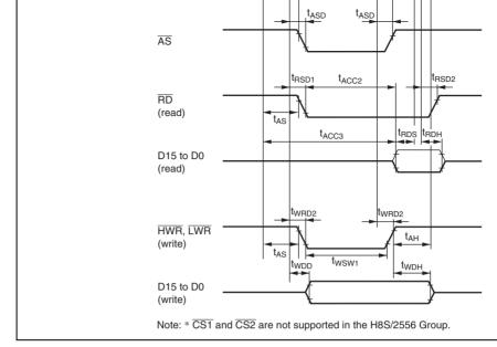
Figure 24.9 Basic Bus Timing: Two-State Access
