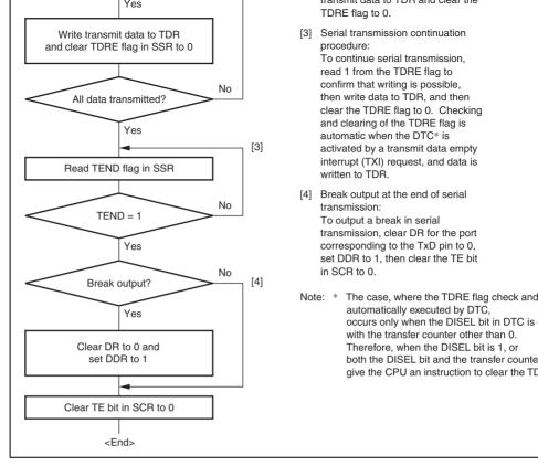
Figure 13.7 Sample Serial Transmission Flowchart
