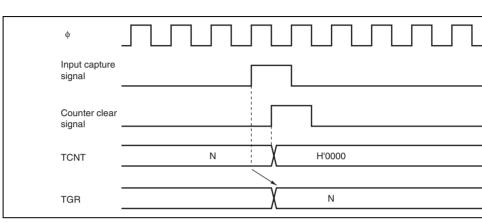
Figure 10.35 Counter Clear Timing (Input Capture)
