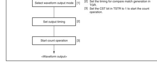
Figure 10.5 Example of Setting Procedure for Waveform Output by Compare I
