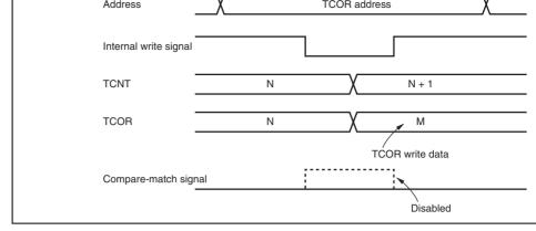
Figure 11.12 Contention between TCOR Write and Compare-Match
