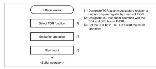
Figure 10.14 Example of Buffer Operation Setting Procedure
