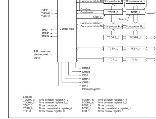
Figure 11.1 Block Diagram of 8-Bit Timer Module
