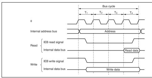
Figure 7.10 On-Chip IEB Module Access Cycle
