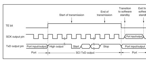
Figure 13.35 Asynchronous Transmission Using Internal Clock
