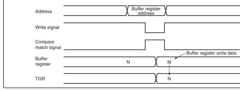
Figure 10.48 Contention between Buffer Register Write and Compare Ma
