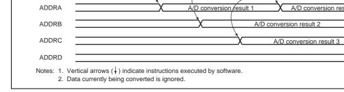
Figure 15.4 A/D Conversion Timing (Scan Mode, Channels AN0 to AN2 Selec
