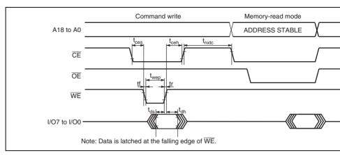
Figure 20.29 Memory Read Timing after Command Programming
