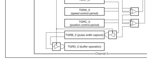
Figure 10.29 Phase Counting Mode Application Example
