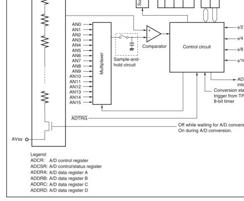
Figure 15.1 Block Diagram of A/D Converter
