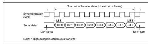
Figure 13.14 Data Format in Clocked Synchronous Communication (For LSB-
