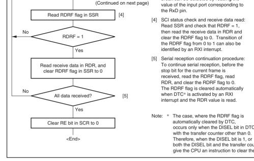
Figure 13.9 Sample Serial Reception Data Flowchart (1)
