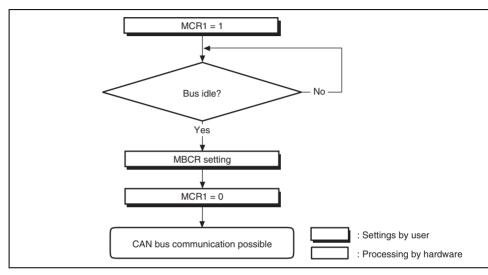
Figure 18.14 HCAN Halt Mode Flowchart
