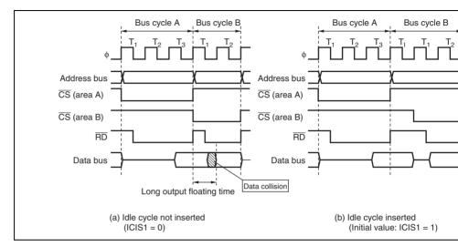
Figure 7.27 Example of Idle Cycle Operation (1)
