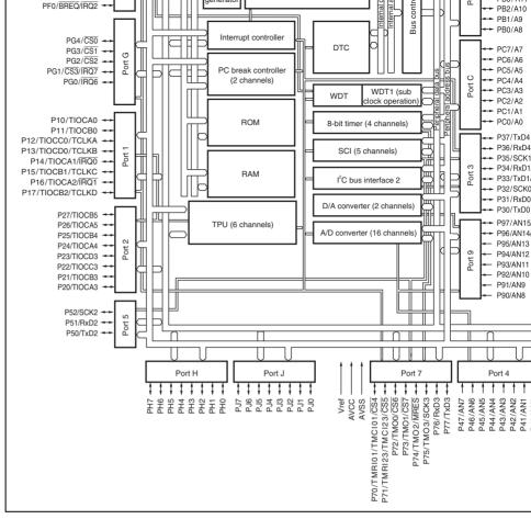
Figure 1.3 Internal Block Diagram of H8S/2506 Group
