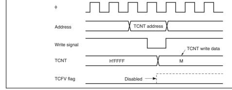
Figure 10.53 Contention between TCNT Write and Overflow
