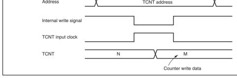
Figure 11.11 Contention between TCNT Write and Increment
