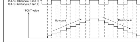
Figure 10.25 Example of Phase Counting Mode 1 Operation
