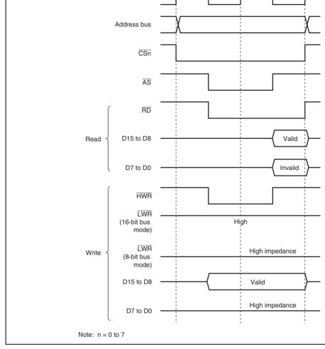
Figure 7.16 Bus Timing for 8-Bit 2-State Access Space
