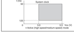
Figure 24.1 (2) Power Supply Voltage and Operating Ranges (H8S/2556 Gro
