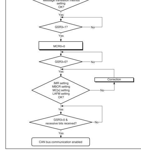
Figure 18.7 Software Reset Flowchart
