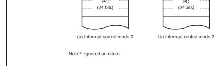
Figure 4.2 Stack State after Exception Handling (Advanced Mode)
