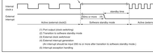
Figure 21.7 External Clock Switching Timing (Examples)
