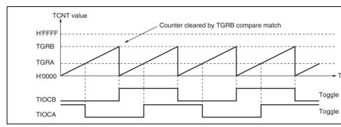
Figure 10.7 Example of Toggle Output Operation
