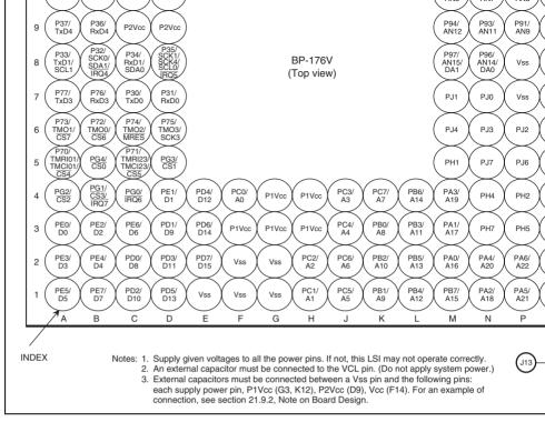
Figure 1.8 Pin Arrangement of H8S/2506 Group (BP-176V)
