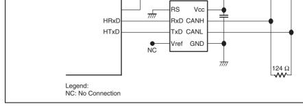
Figure 18.16 High-Speed Interface Using PCA82C250
