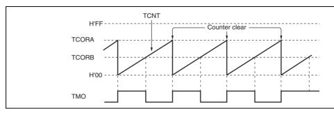
Figure 11.2 Example of Pulse Output
