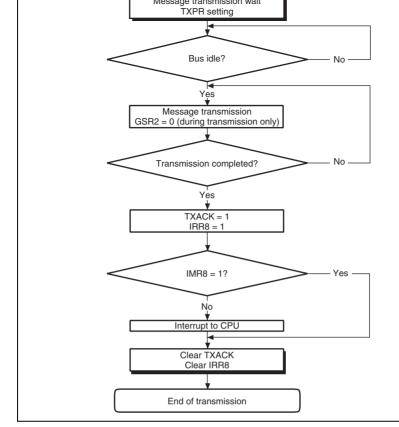
Figure 18.9 Transmission Flowchart
