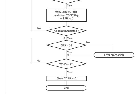
Figure 13.28 Example of Transmission Processing Flow
