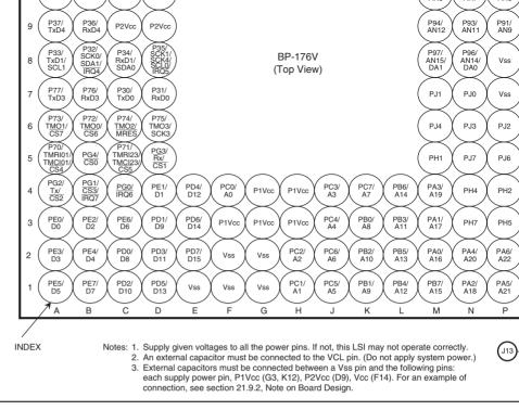
Figure 1.7 Pin Arrangement of H8S/2552 Group (BP-176V)
