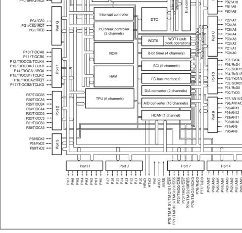
Figure 1.1 Internal Block Diagram of H8S/2556 Group
