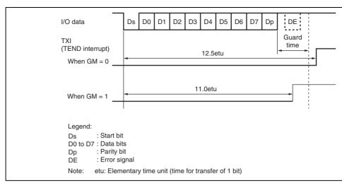
Figure 13.27 TEND Flag Generation Timing in Transmission Operation
