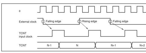
Figure 10.31 Count Timing in External Clock Operation
