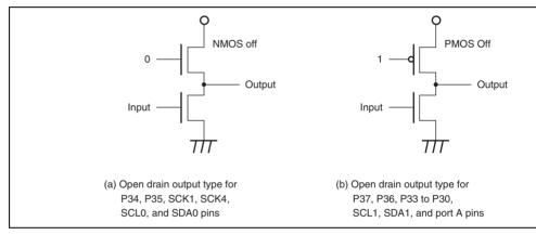
Figure 9.1 Types of Open Drain Outputs
