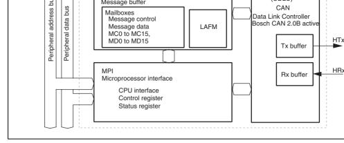
Figure 18.1 HCAN Block Diagram
