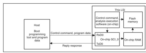
Figure 20.6 System Configuration in Boot Mode
