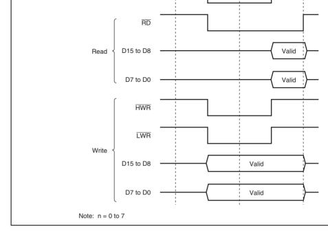
Figure 7.20 Bus Timing for 16-Bit 2-State Access Space (3) (Word Access
