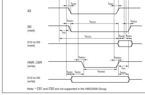
Figure 24.10 Basic Bus Timing: Three-State Access
