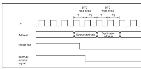
Figure 10.43 Timing for Status Flag Clearing by DTC Activation
