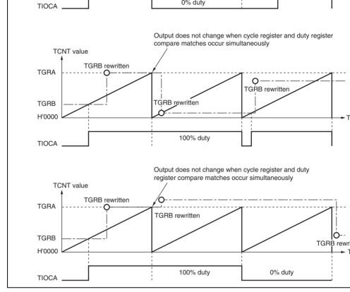
Figure 10.23 Example of PWM Mode Operation (3)
