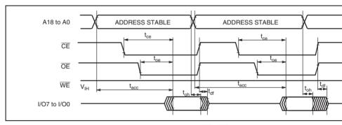
Figure 20.32 Waveform of CE, OE Clock System Read
