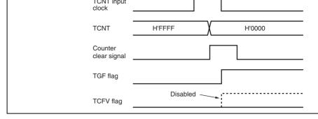
Figure 10.52 Contention between Overflow and Counter Clearing
