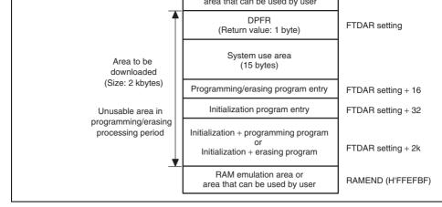
Figure 20.10 RAM Map when Programming/Erasing Is Executed
