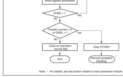
Figure 8.5 Flowchart of DTC Operation
