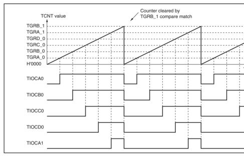
Figure 10.22 Example of PWM Mode Operation (2)
