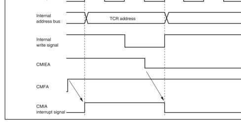
Figure 5.9 Contention between Interrupt Generation and Disabling
