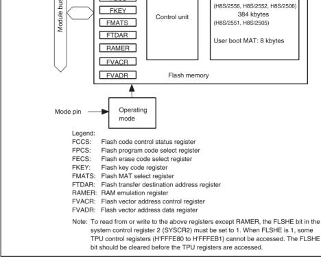
Figure 20.1 Block Diagram of Flash Memory
