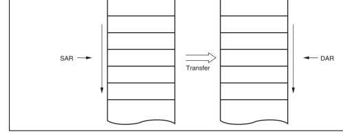
Figure 8.6 Memory Mapping in Normal Mode
