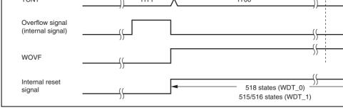
Figure 12.5 Timing of WOVF Setting
