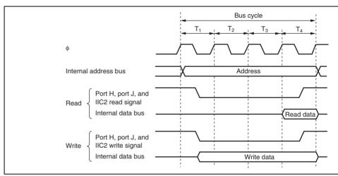
Figure 7.8 On-Chip Port H, Port J, and IIC2 Module Access Cycle
