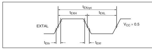
Figure 21.5 External Clock Input Timing
