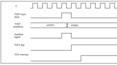
Figure 10.40 TCIV Interrupt Setting Timing
