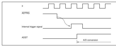
Figure 15.6 External Trigger Input Timing
