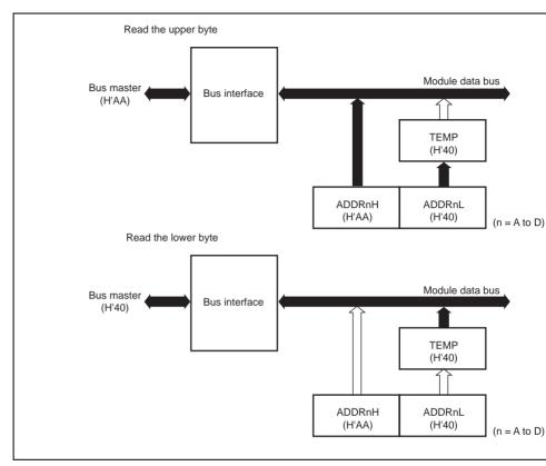
Figure 15.2 shows data flow when accessing to ADDR.
