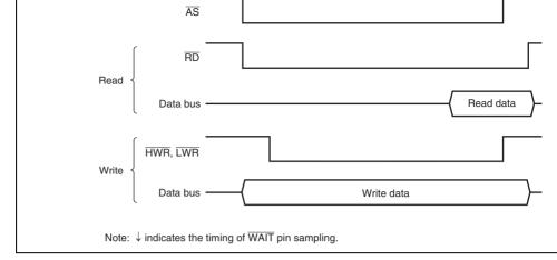
Figure 7.24 Example of Wait State Insertion Timing
