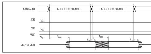
Figure 20.31 Waveform of CE, OE Enable State Read
