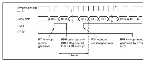
Figure 13.18 Example of SCI Operation in Reception
