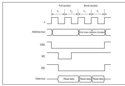
Figure 7.26 Example of Burst ROM Access Timing (When AST0 = BRSTS1 =
