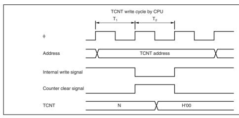
Figure 11.10 Contention between TCNT Write and Clear
