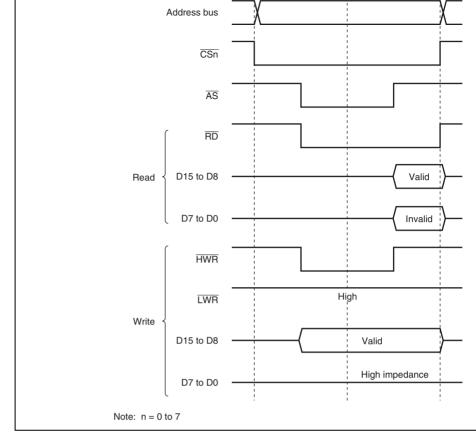
Figure 7.18 Bus Timing for 16-Bit 2-State Access Space (1) (Even Address Byte
