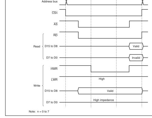
Figure 7.21 Bus Timing for 16-Bit 3-State Access Space (1) (Even Address Byte A
