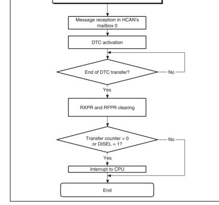
Figure 18.15 DTC Transfer Flowchart
