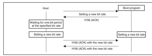
Figure 20.26 New Bit-Rate Selection Sequence
