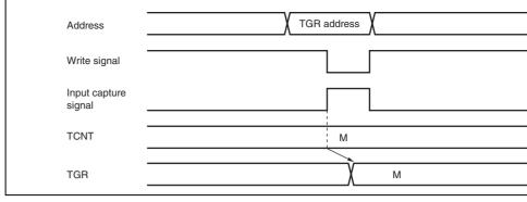
Figure 10.50 Contention between TGR Write and Input Capture
