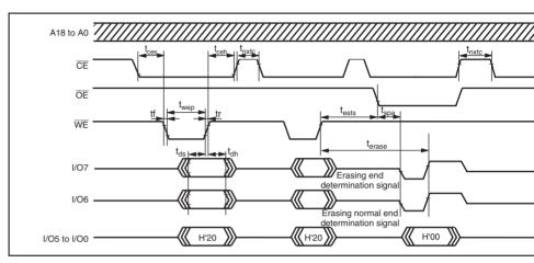
Figure 20.34 Waveform in Auto-Erase Mode
