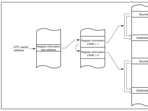
Figure 8.9 Chain Transfer Operation
