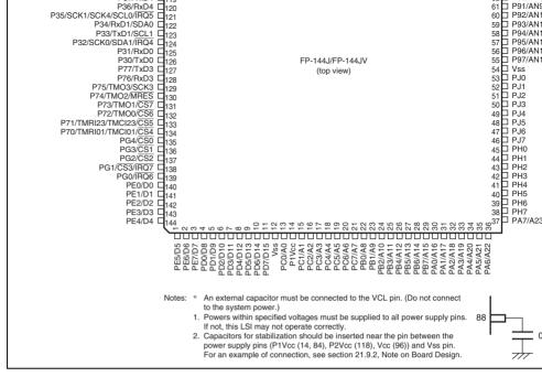
Figure 1.6 Pin Arrangement of H8S/2506 Group (FP-144J and FP-144JV)
