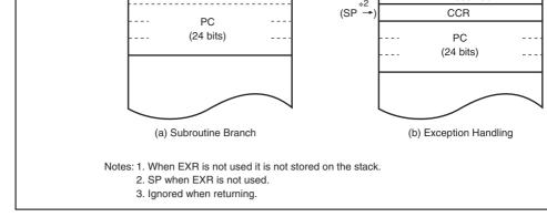
Figure 2.4 Stack Structure in Advanced Mode
