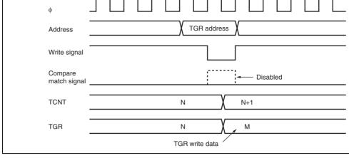
Figure 10.47 Contention between TGR Write and Compare Match
