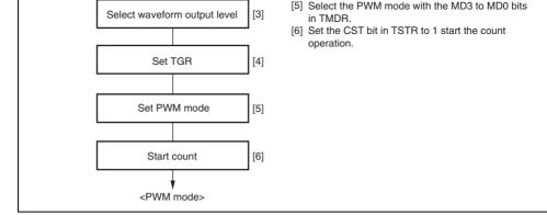
Figure 10.20 Example of PWM Mode Setting Procedure
