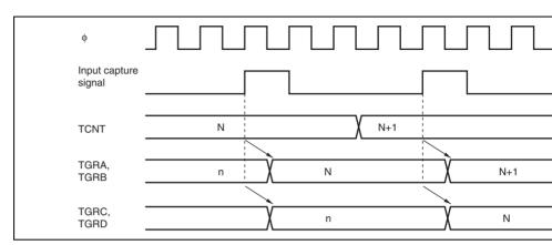
Figure 10.37 Buffer Operation Timing (Input Capture)
