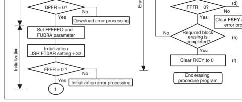
Figure 20.12 Erasing Procedure
