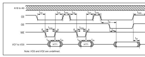
Figure 20.35 Waveform in Status-Read Mode
