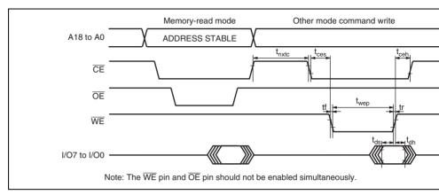
Figure 20.30 Waveform of Transition from Memory-Read Mode to Other Me
