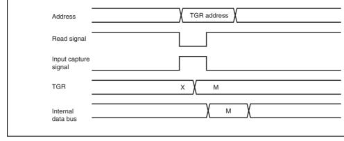
Figure 10.49 Contention between TGR Read and Input Capture
