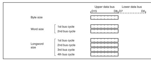
Figure 7.14 Access Sizes and Data Alignment Control (8-Bit Access Spac
