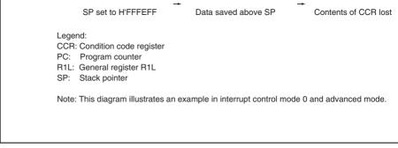
Figure 4.3 Operation when SP Value Is Odd
