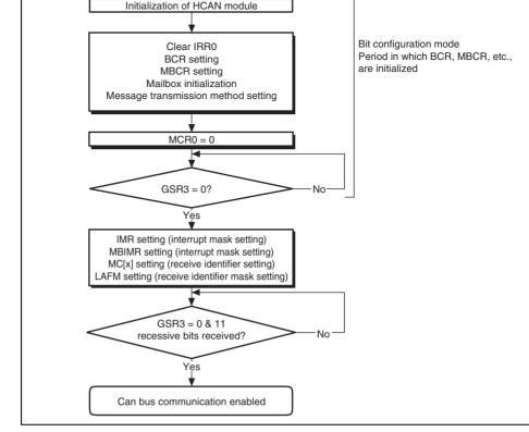
Figure 18.6 Hardware Reset Flowchart
