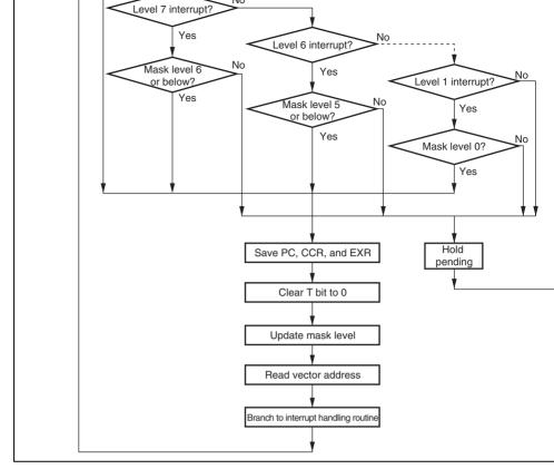
Figure 5.6 Flowchart of Procedure up to Interrupt Acceptance in Interrupt Control Mode 2
