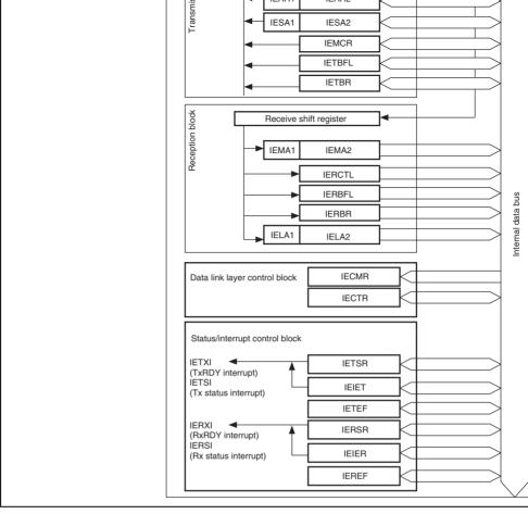
Figure 17.1 Block Diagram of IEB
