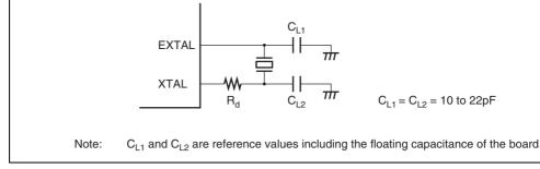
Figure 21.2 Connection of Crystal Resonator (Example)
