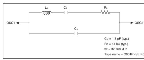
Figure 21.9 Equivalent Circuit for 32.768-kHz Crystal Resonator
