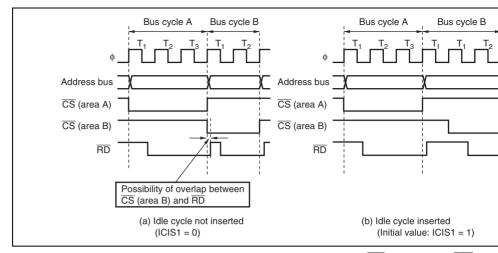
Figure 7.29 Relationship between Chip Select ( $\overline{CS}$ ) and Read ( $\overline{RD}$ )
