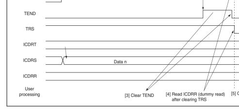
Figure 14.10 Slave Transmit Mode Operation Timing (2)
