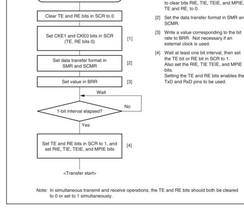
Figure 13.15 Sample SCI Initialization Flowchart
