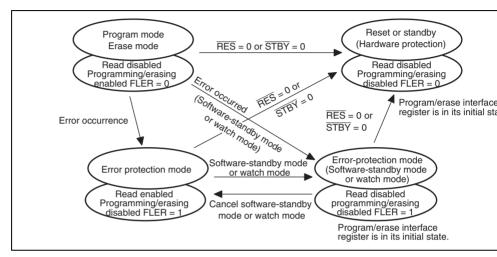
Figure 20.16 Transitions to Error-Protection State
