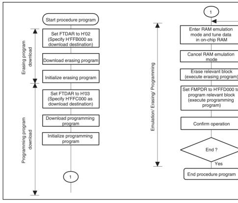
Figure 20.13 Sample Procedure of Repeating RAM Emulation, Erasing, and Prog (Overview)
