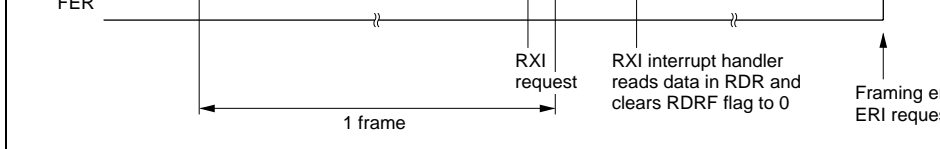
Figure 13.8 Example of SCI Receive Operation (8-Bit Data with Parity and One Stop Bit)
