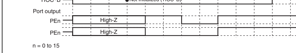
Figure 10.141 Error Occurrence in PWM Mode 1, Recovery in Normal Mode
