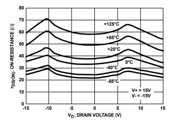
FIGURE 7. rDS(ON) vs VD AND TEMPERATURE
