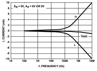
FIGURE 14. SUPPLY CURRENTS vs SWITCHING FREQUENCY
