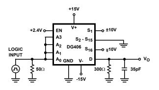
FIGURE 3A. DG406 TEST CIRCUIT
