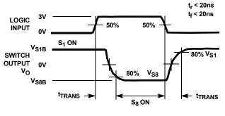
FIGURE 3C. MEASUREMENT POINTS FIGURE 3. TRANSITION TIME
