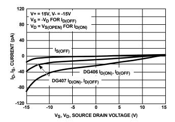
FIGURE 9. ID, IS LEAKAGE CURRENTS VS ANALOG VOLTAGE
