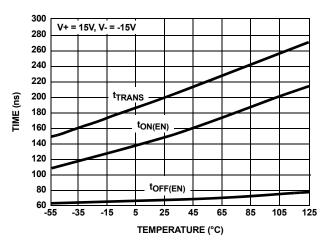
FIGURE 15.  $t_{ON}/t_{OFF}$  vs TEMPERATURE
