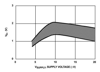
FIGURE 16. SWITCHING THRESHOLD vs SUPPLY VOLTAGE
