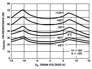
FIGURE 2. ±15 DUAL SUPPLY r<sub>on</sub> curves at various temperatures
