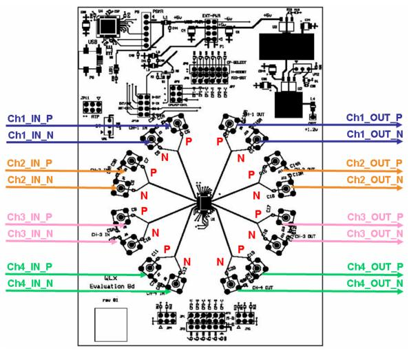
FIGURE 5. QLX4600-S30 EVALUATION BOARD RF-I/O INTERFACE
