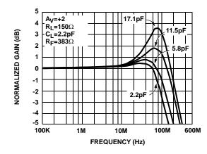
FIGURE 3. GAIN vs FREQUENCY FOR VARIOUS CIN-
