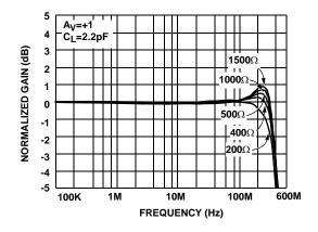
FIGURE 8. GAIN vs FREQUENCY FOR VARIOUS RL
