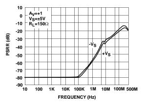
FIGURE 13. PSRR vs FREQUENCY
