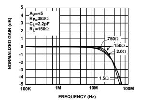
FIGURE 7. GAIN vs FREQUENCY FOR VARIOUS RL
