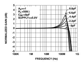
FIGURE 2. GAIN vs FREQUENCY FOR VARIOUS  $C_{L}$
