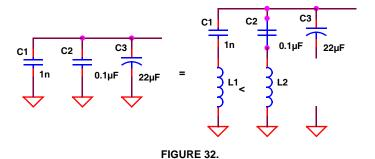
Above its serial resonance C2\* the ideal capacitance of C2 is a short, the Tantalum capacitor for high frequencies is not effective, the left over is C1 capacitor and L1 + L2 inductors, we get a parallel tank circuit, which is at it's resonance a high impedance path and do not carry any high frequency current, it does not work as bypass at all!
