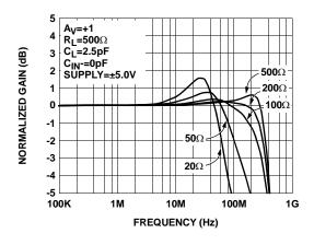
FIGURE 6. GAIN vs FREQUENCY FOR VARIOUS RL
