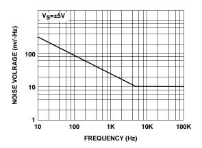
FIGURE 10. EQUIVALENT INPUT VOLTAGE NOISE vs FREQUENCY
