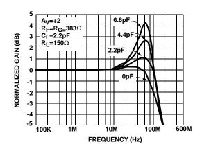
FIGURE 4. GAIN vs FREQUENCY FOR VARIOUS CIN-
