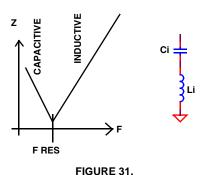
The capacitor will behave as a capacitor up to its resonance frequency, above the resonance frequency it will behave as an inductor.
