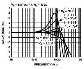
FIGURE 4. FREQUENCY RESPONSE vs CL
