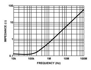
FIGURE 9. OUTPUT IMPEDANCE vs FREQUENCY
