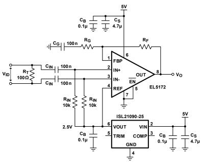
FIGURE 26. Single Supply Operation
