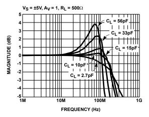
FIGURE 5. FREQUENCY RESPONSE vs CL
