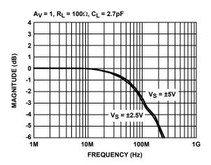
FIGURE 2. FREQUENCY RESPONSE vs SUPPLY VOLTAGE
