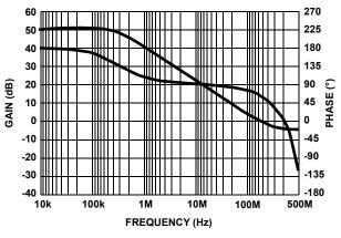
FIGURE 8. OPEN LOOP GAIN
