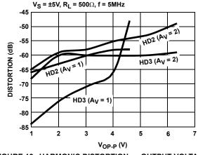
FIGURE 13. HARMONIC DISTORTION vs OUTPUT VOLTAGE
