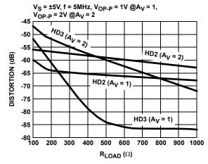
FIGURE 14. HARMONIC DISTORTION vs LOAD RESISTANCE
