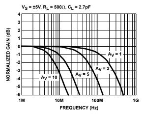
FIGURE 3. FREQUENCY RESPONSE vs VARIOUS GAIN
