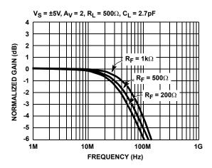
FIGURE 6. FREQUENCY RESPONSE FOR VARIOUS RF
