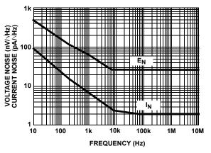
FIGURE 12. VOLTAGE AND CURRENT NOISE vs FREQUENCY
