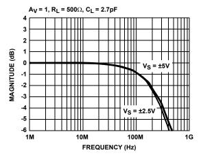
FIGURE 1. FREQUENCY RESPONSE vs SUPPLY VOLTAGE
