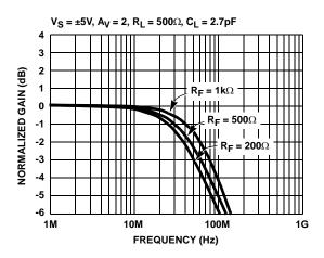
FIGURE 6. FREQUENCY RESPONSE FOR VARIOUS RF
