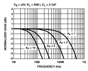
FIGURE 3. FREQUENCY RESPONSE vs VARIOUS GAIN
