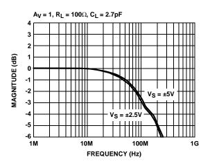
FIGURE 2. FREQUENCY RESPONSE vs SUPPLY VOLTAGE
