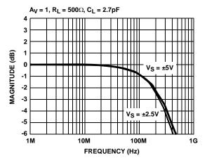
FIGURE 1. FREQUENCY RESPONSE vs SUPPLY VOLTAGE
