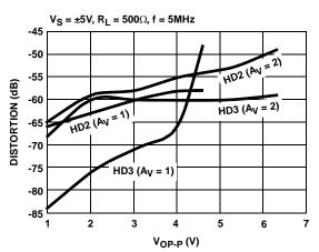
FIGURE 14. HARMONIC DISTORTION vs OUTPUT VOLTAGE
