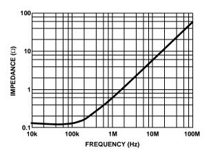
FIGURE 9. OUTPUT IMPEDANCE vs FREQUENCY
