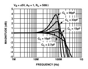
FIGURE 5. FREQUENCY RESPONSE vs CL
