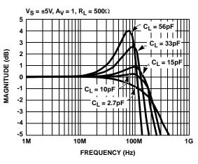
FIGURE 4. FREQUENCY RESPONSE vs CL
