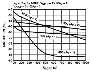
FIGURE 15. HARMONIC DISTORTION vs LOAD RESISTANCE
