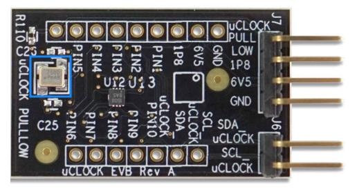
Figure 7. 5L1503 Evaluation Board (board populated with a 25MHz crystal)
