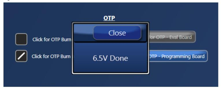
Step 3. Once the previous step is completed, a new window will pop-up confirming to proceed with the OTP burn. Please note that this process cannot be reverted back.
