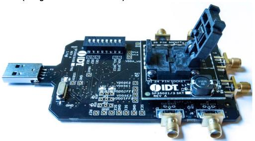
Connect the USB board along with the socket board as shown above. Please, note that the blank part can only be burnt using the socket board. The part on the programming board is used for the purpose of validation. Once, the validation is complete, the user needs to connect the socket board to burn the part. The socket board supports two types of packages: 20 and 24 pins. The following description and images are restricted to 24 PIN socket board.
