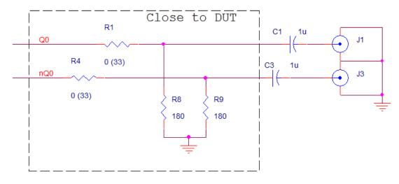
\* If the output frequency is below 50MHz, increase the value of C1 and C3.
