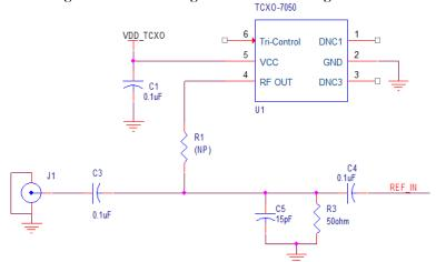
Figure 11. External Signal Reference Configuration
