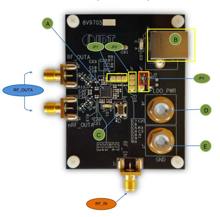
Figure 1. Evaluation Board Top View
