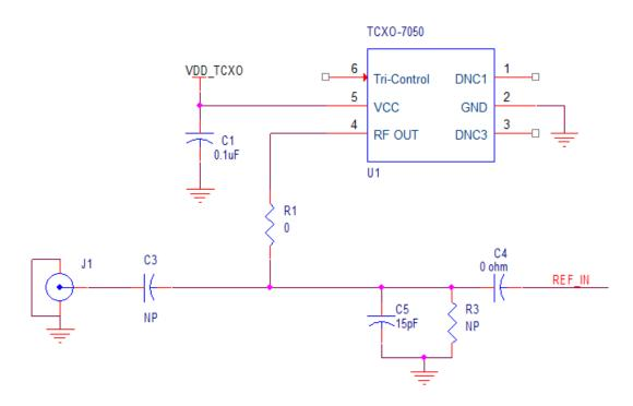
**Figure 4. Output Termination Schematic**
