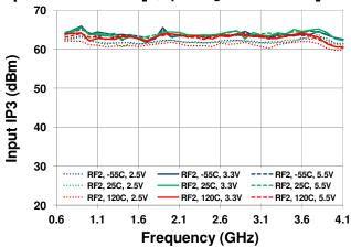
Input IP3 RF2 Port [Tc operating = -40C to 105C]
