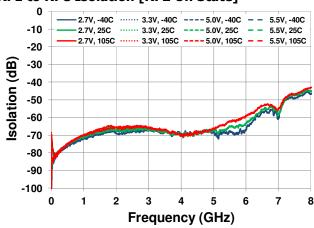
RF2 to RFC Isolation [RF1 On State]
