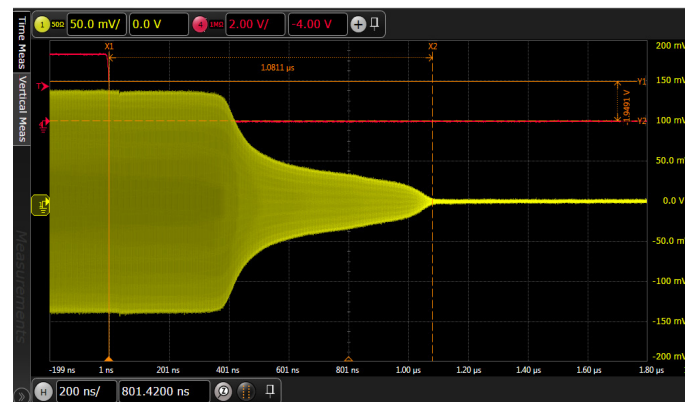
Figure 25. Switching Time [Insertion Loss to Isolation State]
