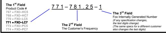
This example, FXO-LC736R-781.25 = LVDS Output, Ceramic, 7 x 5mm Package, 3.3V, ±25 PPM Stability, -40 to +85°C Temperature Range, at 781.25 MHz
