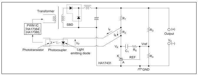
Figure 2 Typical Shunt Regulator/Error Amplifier
