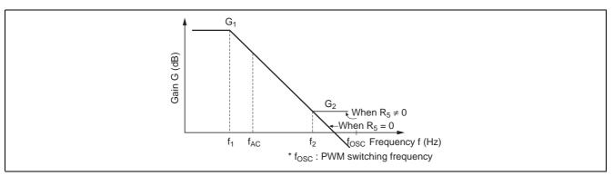
Figure 3 HA17431 Error Amplification Characteristic
