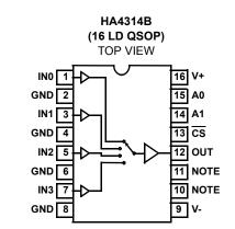
NOTE: These pins must be left floating or connected to ground
