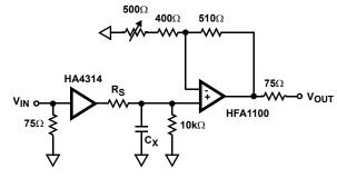
NOTE:  $C_L = C_X + Test$  Fixture Capacitance.
