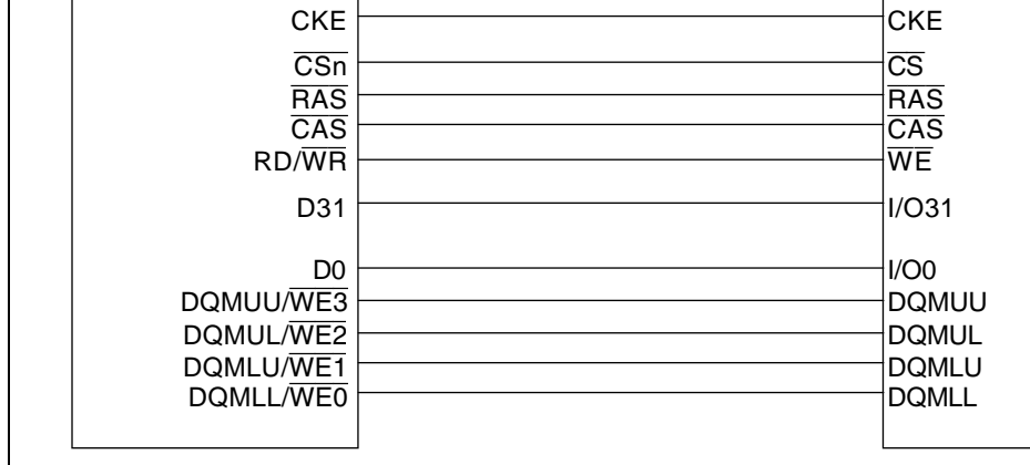
Figure 7.4 256 Mbit Synchronous DRAM (8 Mword × 32 bit) Connection Example
