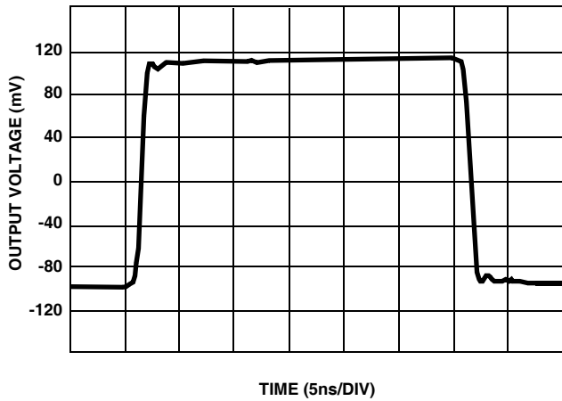
FIGURE 1. SMALL SIGNAL PULSE RESPONSE
