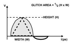
FIGURE 2. OUTPUT SETTLING TIME DIAGRAM
