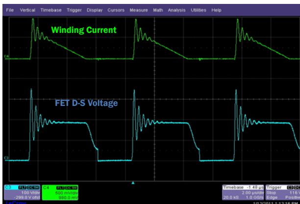
FIGURE 14. QUASI-RESONANT NEAR-ZVS SWITCHING
