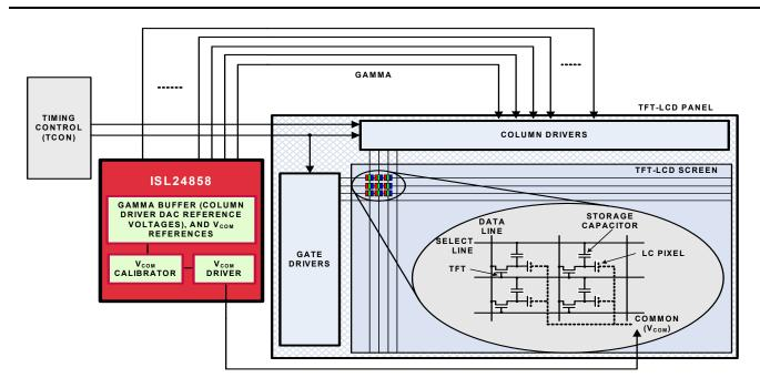
FIGURE 1. TYPICAL APPLICATION: TFT-LCD REFERENCE VOLTAGE GENERATOR
