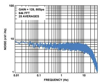
FIGURE 22. NOISE DENSITY vs FREQUENCY AT GAIN = 128, 80Sps
