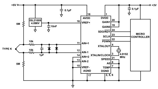
FIGURE 39. THERMOCOUPLE MEASUREMENT APPLICATION
