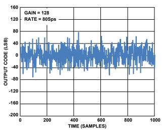
FIGURE 16. NOISE AT GAIN = 128, 80Sps
