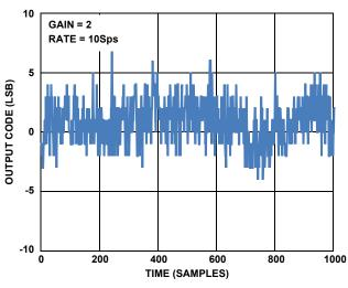
FIGURE 4. NOISE AT GAIN = 2, 10Sps
