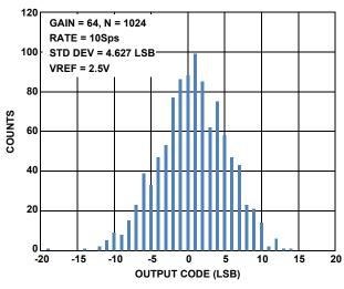
FIGURE 7. NOISE HISTOGRAM AT GAIN = 64, 10Sps
