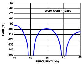
FIGURE 27. 10Sps: 50/60Hz NOISE REJECTION, 45Hz TO 65Hz
