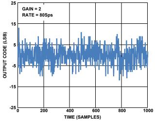
FIGURE 12. NOISE AT GAIN = 2, 80Sps
