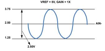
FIGURE 23. DIFFERENTIAL INPUT FOR VREF = 5V, GAIN = 1X
