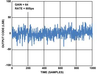
FIGURE 14. NOISE AT GAIN = 64, 80Sps
