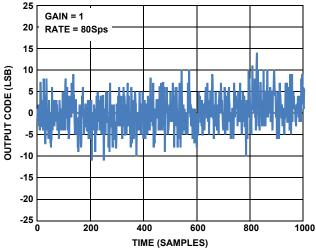
FIGURE 10. NOISE AT GAIN = 1, 80Sps
