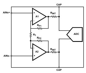
FIGURE 24. SIMPLIFIED PROGRAMMABLE GAIN AMPLIFIER BLOCK DIAGRAM
