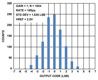
FIGURE 3. NOISE HISTOGRAM AT GAIN = 1, 10Sps
