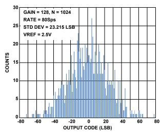
FIGURE 17. NOISE HISTOGRAM AT GAIN = 128, 80Sps
