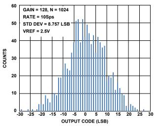
FIGURE 9. NOISE HISTOGRAM AT GAIN = 128, 10Sps
