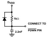
FIGURE 36. PDWNDELAY CIRCUIT
