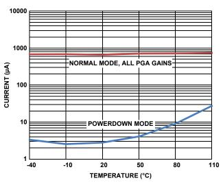
FIGURE 19. DIGITAL CURRENT vs TEMPERATURE
