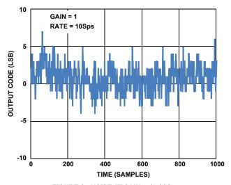
FIGURE 2. NOISE AT GAIN = 1, 10Sps
