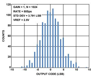
FIGURE 11. NOISE HISTOGRAM AT GAIN = 1, 80Sps
