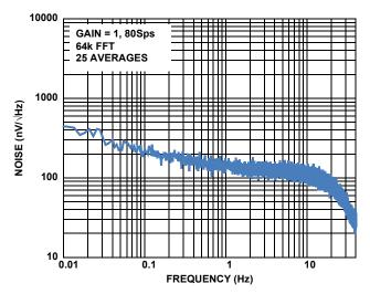
FIGURE 21. NOISE DENSITY vs FREQUENCY AT GAIN = 1, 80Sps
