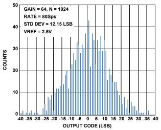
FIGURE 15. NOISE HISTOGRAM AT GAIN = 64, 80Sps
