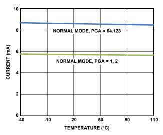
FIGURE 18. ANALOG CURRENT vs TEMPERATURE
