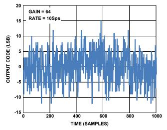
FIGURE 6. NOISE AT GAIN = 64, 10Sps
