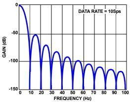
FIGURE 26. 10Sps: FREQUENCY RESPONSE OUT TO 100Hz
