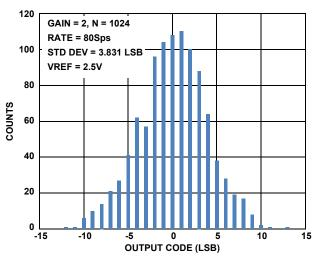
FIGURE 13. NOISE HISTOGRAM AT GAIN = 2, 80Sps
