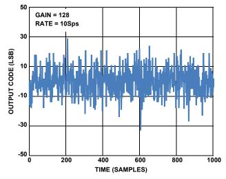
FIGURE 8. NOISE AT GAIN = 128, 10Sps
