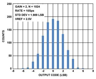
FIGURE 5. NOISE HISTOGRAM AT GAIN = 2, 10Sps
