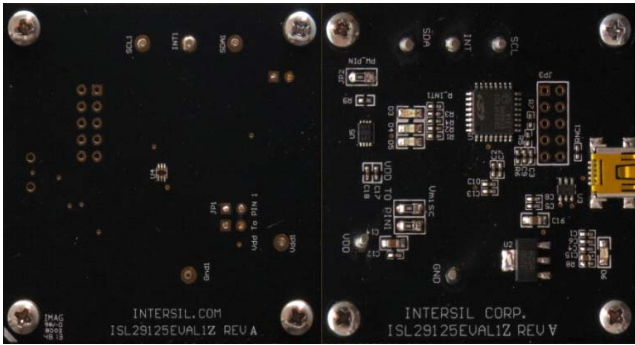
FIGURE 7. ISL29125 EVALUATION BOARD
