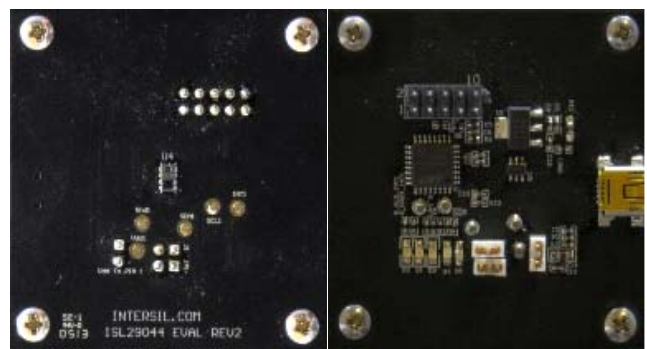
FIGURE 10. ISL29044 EVALUATION BOARD
