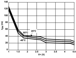
FIGURE 17. INHIBIT TURN - ON TIME vs SUPPLY VOLTAGE
