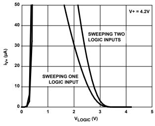
FIGURE 13. I+ CURRENT vs LOGIC VOLTAGE
