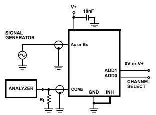
Off-Isolation is measured between COM and "Off" NO terminal on each switch. Signal direction through switch is reversed and worst case values are recorded.
