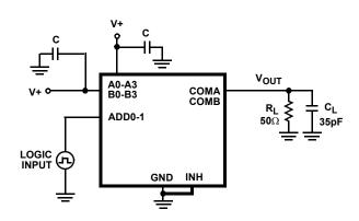
Repeat test for other switches.  $\mathsf{C}_{\mathsf{L}}$  includes fixture and stray capacitance.
