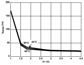
FIGURE 16. ADDRESS TRANS TIME vs SUPPLY VOLTAGE
