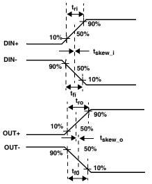
FIGURE 7A. MEASUREMENT POINTS
