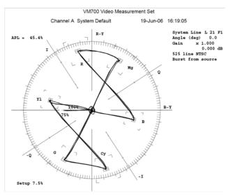
FIGURE 8. VECTOR-SCOPE PLOT BEFORE SWITCH
